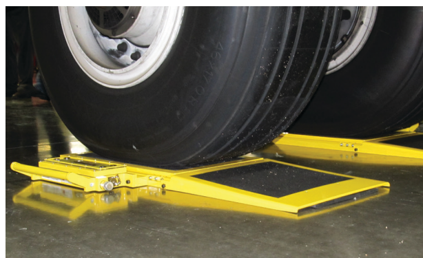
Low-profile scales are certified intrinsically safe for use in hangars.
